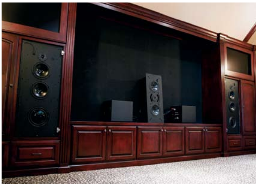
THE CUSTOM-BUILT WALL UNIT holds the James Loudspeakers left and right front speakers, the Samsung LCD HDTVs, and the Screen Research screen, which conceals the center speaker and two 10-inch subwoofers.
